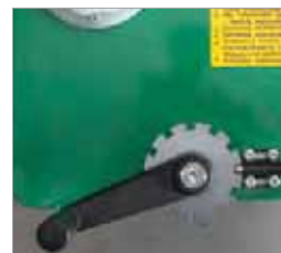
● Smooth depth regulator easy to adjust.
