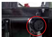
● Warning buzzer for dust collection bag full 2
