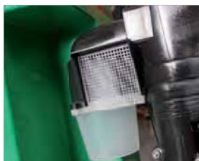
● Cyclone cleaner increase life of engines SHARKY 400/500.
