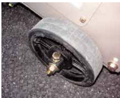
Differential Lock Mechanism The rear wheels are equipped with a differential lock mechanism for better straight-line stability. (MCD-210 series)
