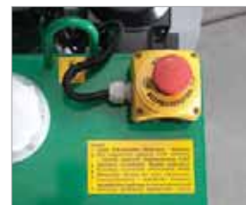
● Safety switch and blade's cover sensor increasing safety work for operator
