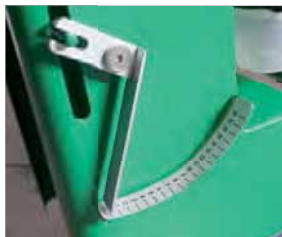
● Depth cutting indicator allow constant checking of cutting depth.
